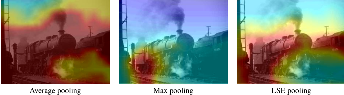
Figure 5. Heat map for class train generated by proposal network trained with average pooling, max pooling and LSE pooling respectively.
